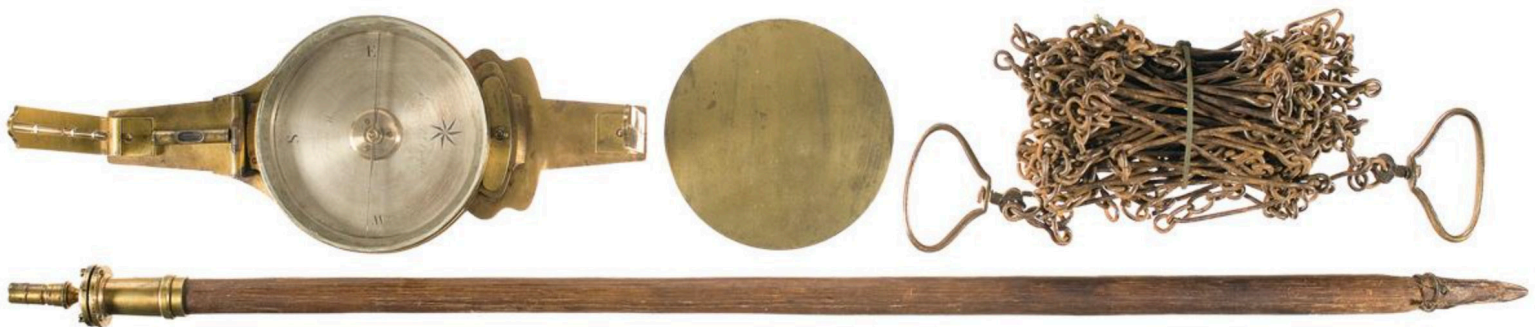
MID-19TH CENTURY SURVEYOR'S CIRCUMFERENTOR, STAFF, AND MEASURING CHAIN
